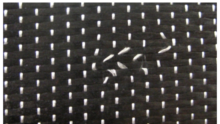
Typical defect which is easily overlooked during manual inspection: Shifted warp thread in a carbon fibre textile.
